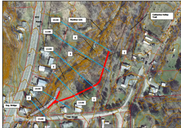
EXHIBIT #9: SITE IMPROVEMENT PLAN Compacted Earth Diversion Berm Project Town of Veteran, Chenango County, New York
